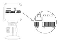
Turn the power switch to "ON", the mode switch button to "DV", and insert a TF card for 24 hours of continuous recording.
