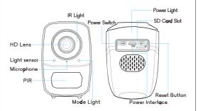
How to factory reset: When the camera is turned on, press and hold the reset button for about 3 seconds until the blue light and green light flash alternately slowly.
