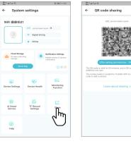
Enter the "Settings" interface of the camera and select "Share" to generate the device sharing QR code. Other users open the APP, click the "Add" button on the home page, and then scan the QR code to add the device.
